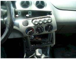
Remove the 2 Torx Screws from the stereo opening(on the uppper edge- no photo)
