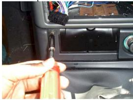
First remove 2 Torx Screws from the underside of the Headlight/dimmer Panel
