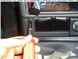
At this point you should be able to pull the Headlight Knob/dimmer Dash Piece and the Piece to the right of the steering
